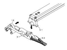
Press the unlocking plate (5.1) downwards with one hand and place the runner (1.0) onto the guide rail (2.0) with the other. The runner can now move freely on the guide rail (2.0).
