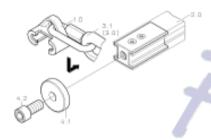
Remove the stop plate (4.1) by detaching the screw (4.2). Insert the runner (1.0) into the guide rail "Söll-MultiRail" (2.0). Hereinafter, fix the stop plate (4.1) again by means of the screw (4.2), to avoid accidental gliding out of the runner. Now, the runner can be moved freely on the remove the . guide rail (1.1). To detach the runner, screw out the stop plate (4.1) and remove the runner from the rail. Finally, fix the stop plate again by means of the screw.
